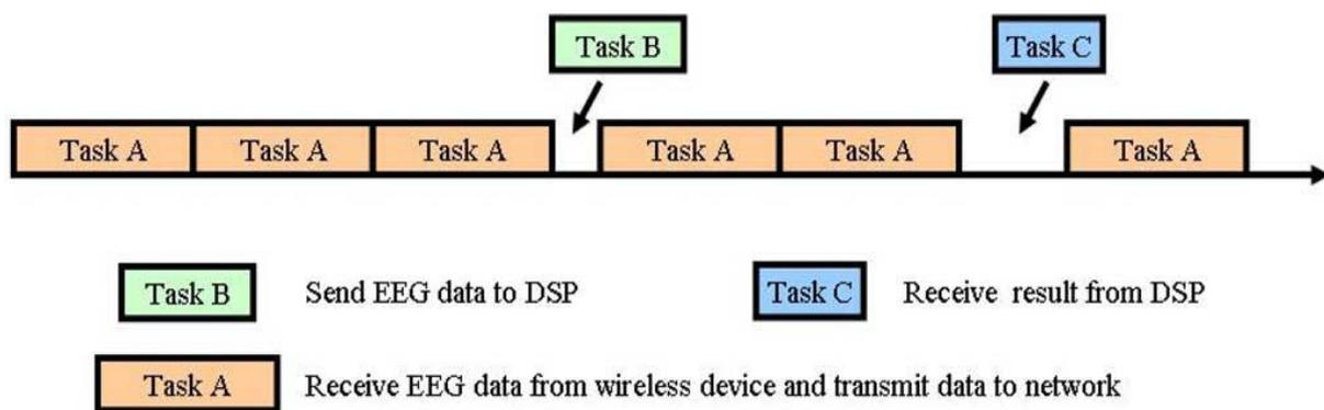
Fig..4. Time series diagram of multitask scheduling mechanism
