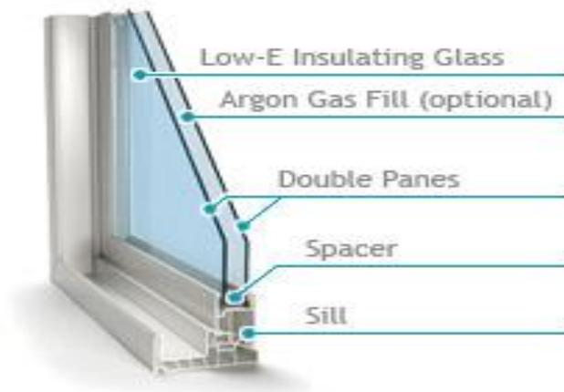
Figure 3:- Double glazed window (structure)
