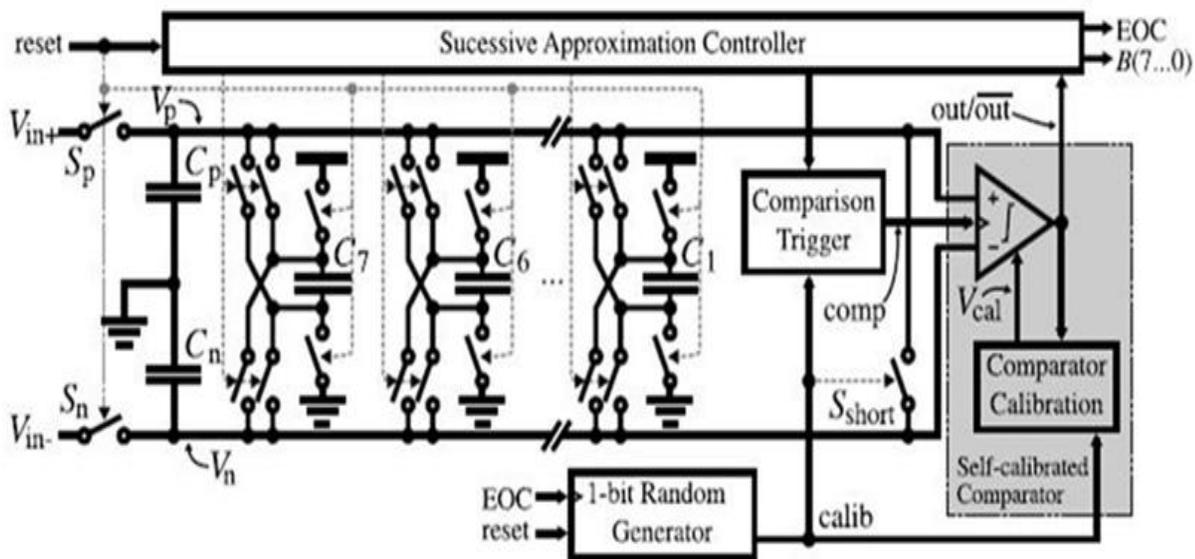
Fig.1. shows the DAC SAR A/D architecture utilizing the proposed self-calibration method in the sampling phase.
