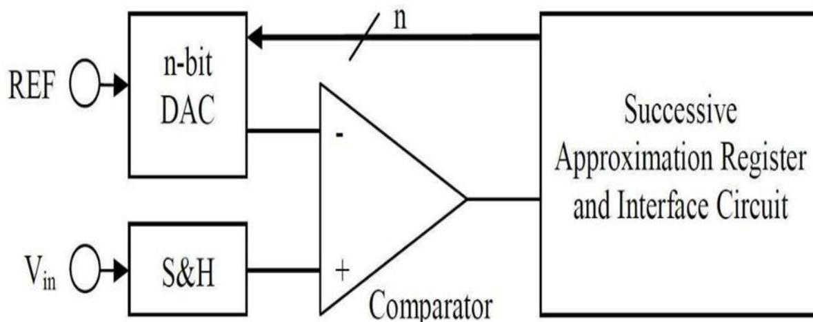
Fig.2. Block Diagram of Conventional SAR A/D Converter
