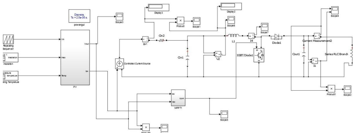
Fig. 8 Model of PV system with MPPT algorithm
