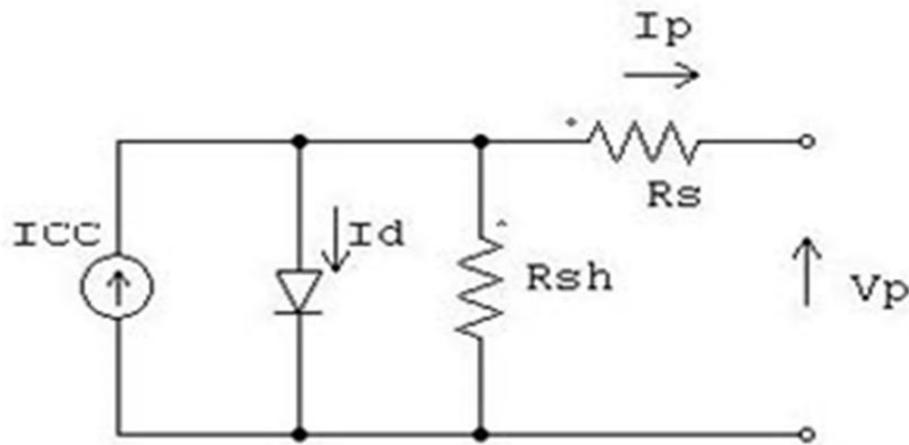
Fig 1: Equivalent Solar Cell Model
