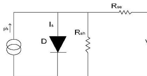
Fig.5 Solar Cell single diode model
