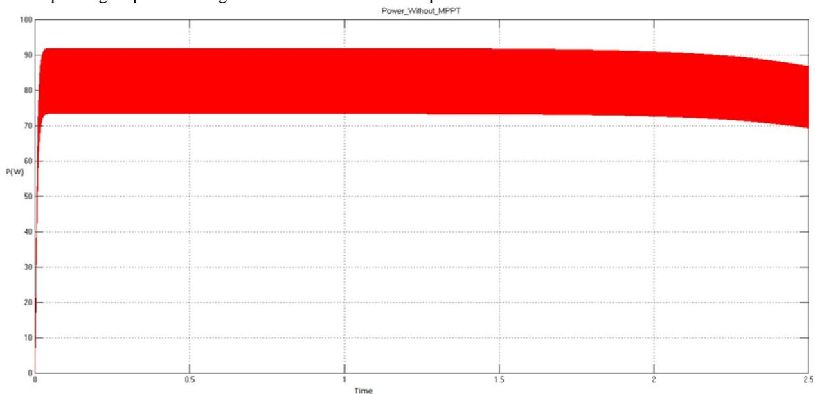
Fig.12, Graph between output power (watt) & time (second) of module at load terminals without MPPT
