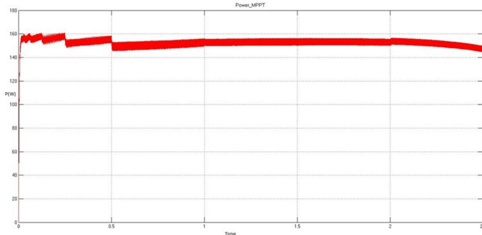
Fig15: Graph between output power (watt) &time (second) of module with MPPT
