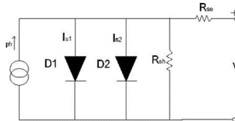
Fig.6 Solar Cell double diode model
