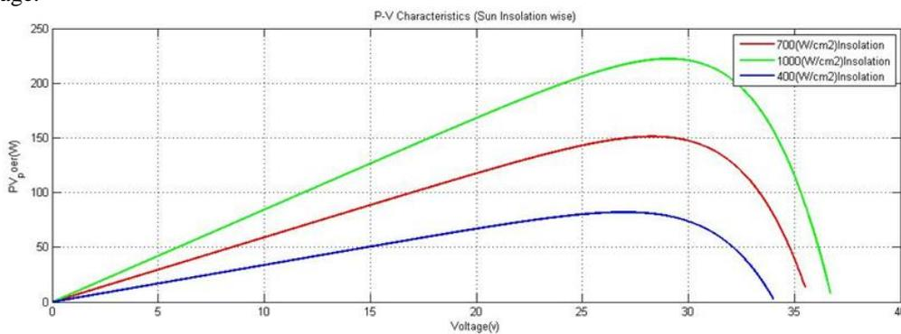
Fig. 4 P-V Curves of Different Sun Irradiation
