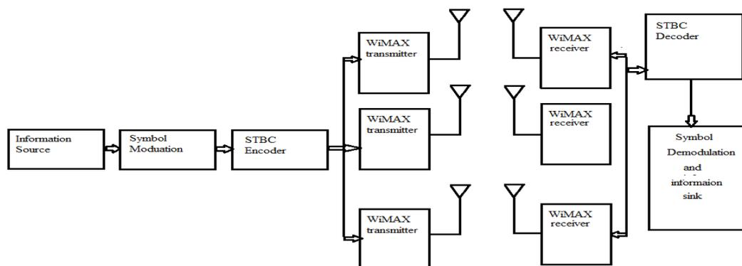
Fig. 5 MIMO-mobile WiMAX model
