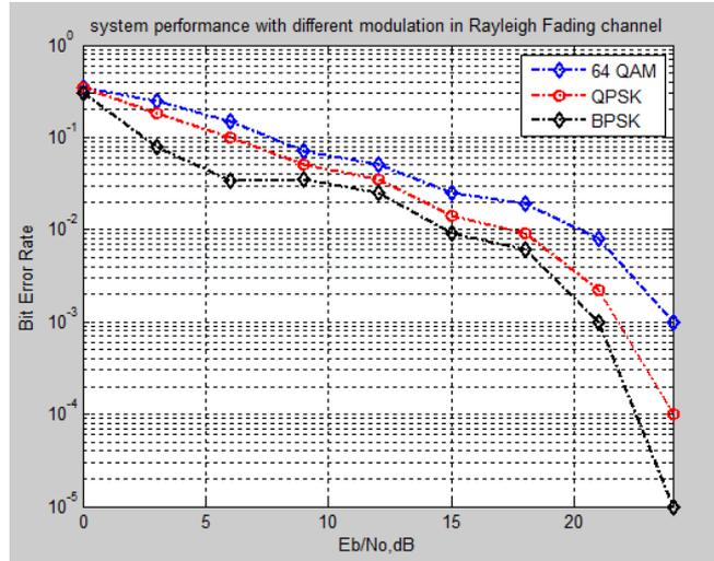
**Fig. 7 BER of MIMO-WiMAX system for different modulation with in Rayleigh Fading channel**
