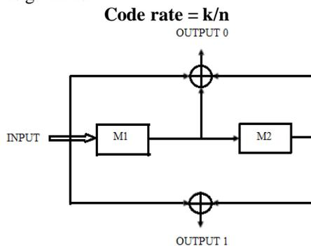
Fig. 2 Convolution Encoder; code rate=1/2, m=2
