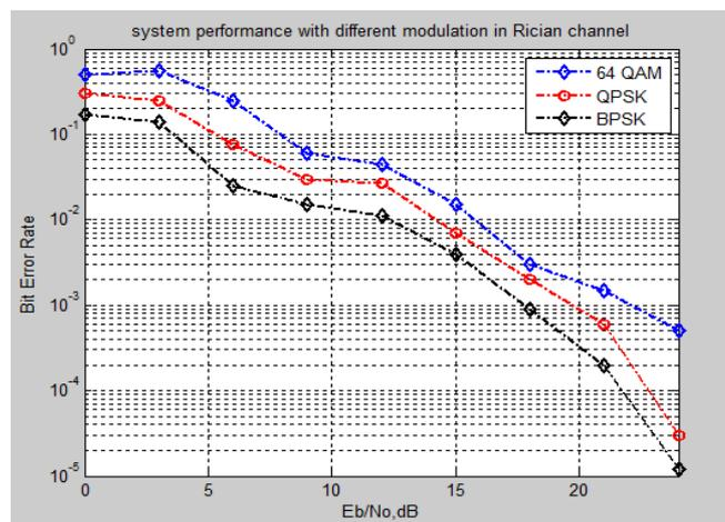
**Fig. 8 BER of MIMO-WiMAX system for different modulation with in Rician channel**
