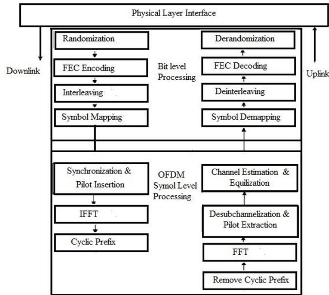
Fig. 1 WiMAX OFDM physical layer model
