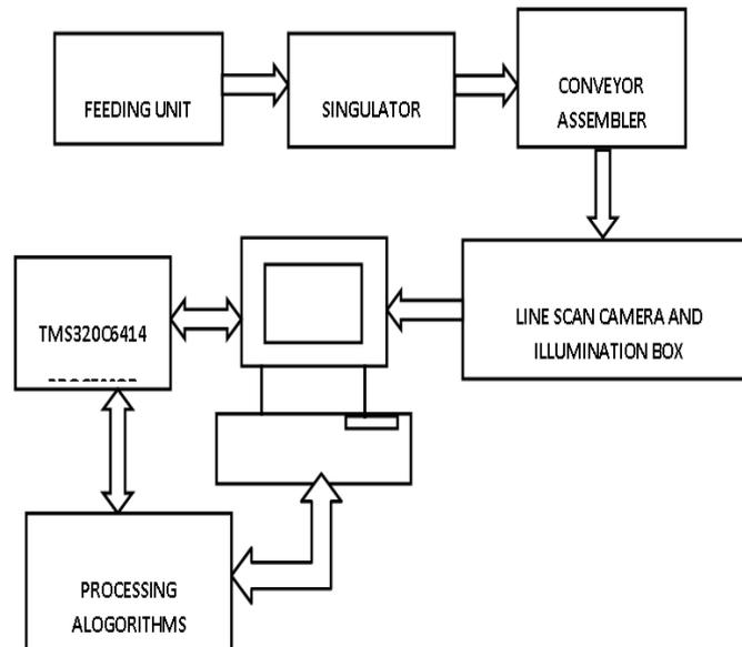
One of the components of the machine vision system for the apple sorting and grading system is the PC platform which acts as the host and a software which is used for inspection [10]. The overall working of this application which would interact with the user and which has been simulated in this project is given below.
