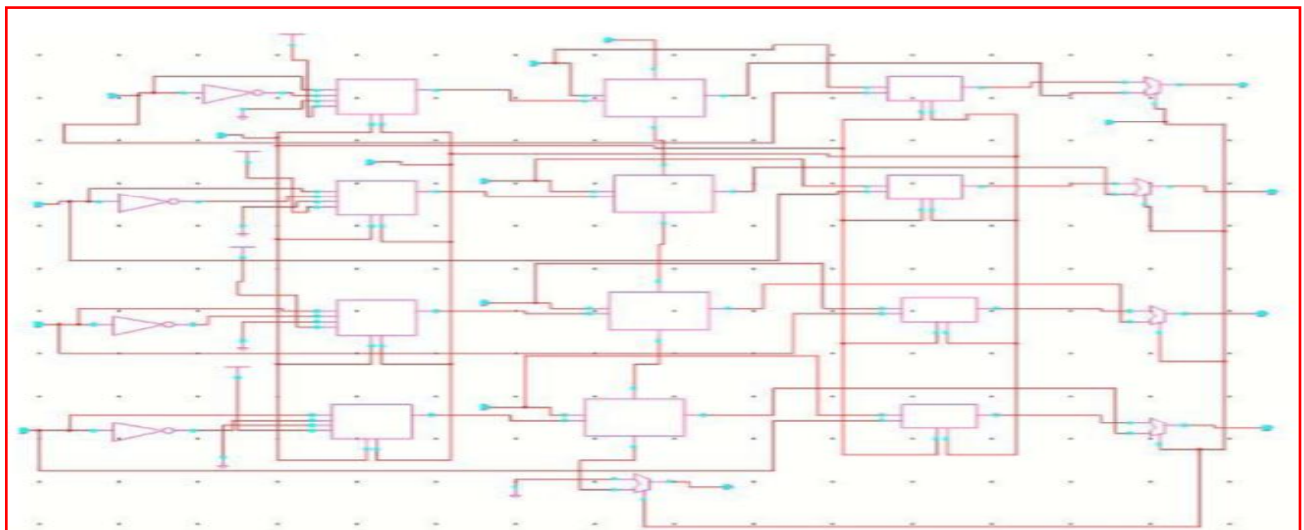
Fig(b): Implementation of 4-bit ALU based on GDI
