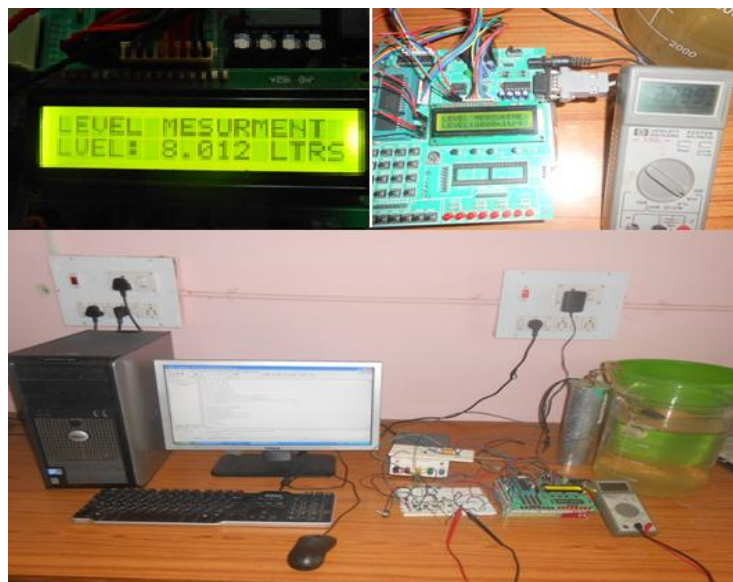
Photograph 1: Liquid Level measurement with float sensor.
