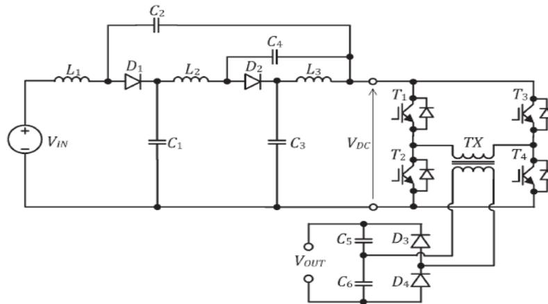
Fig. 3 Front end high step up conversion
