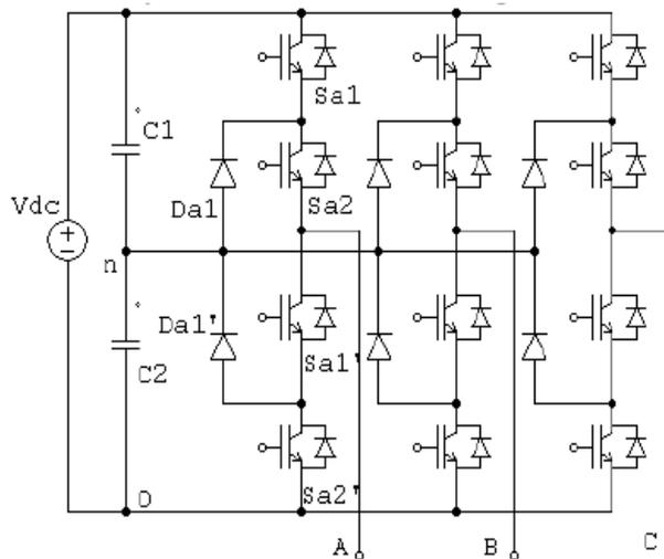
Fig. 6 diode clamped 3-phase, 3-level inverter
