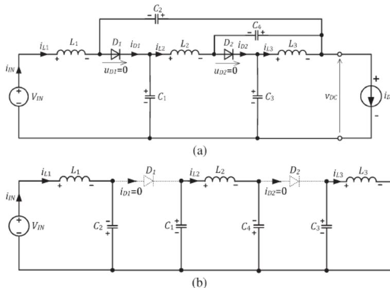
Fig. 4 Equivalent circuits of the cascaded qZS-network:
