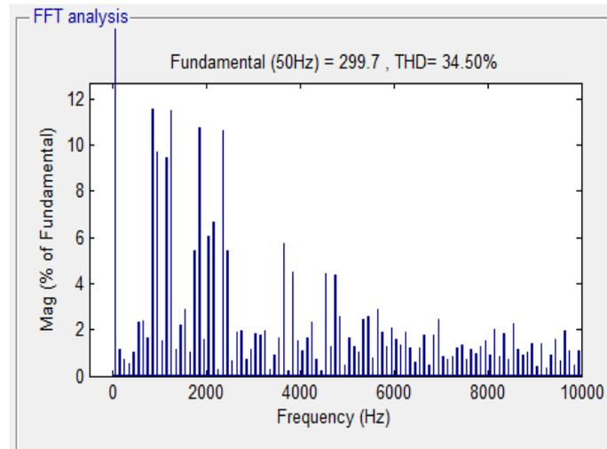
Fig. 12 FFT analysis of inverter output voltage without filters
