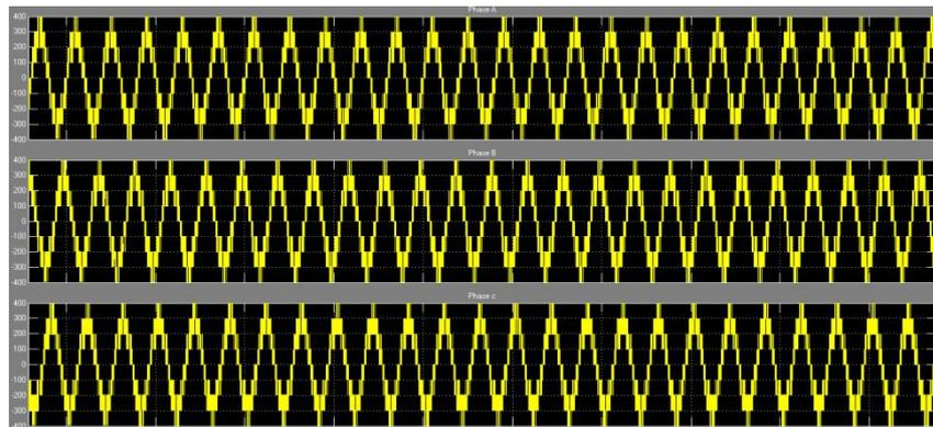
Fig. 11 Inverter output voltage wave forms without filters
