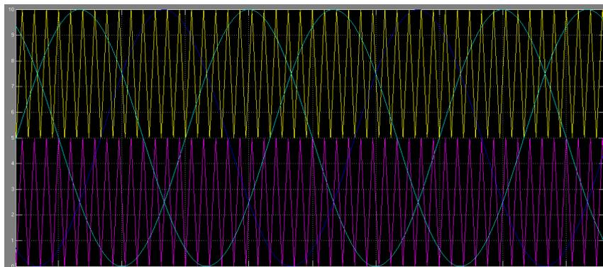
Fig. 10 Sine-Triangular Comparison of 3 level diode clamped inverter
