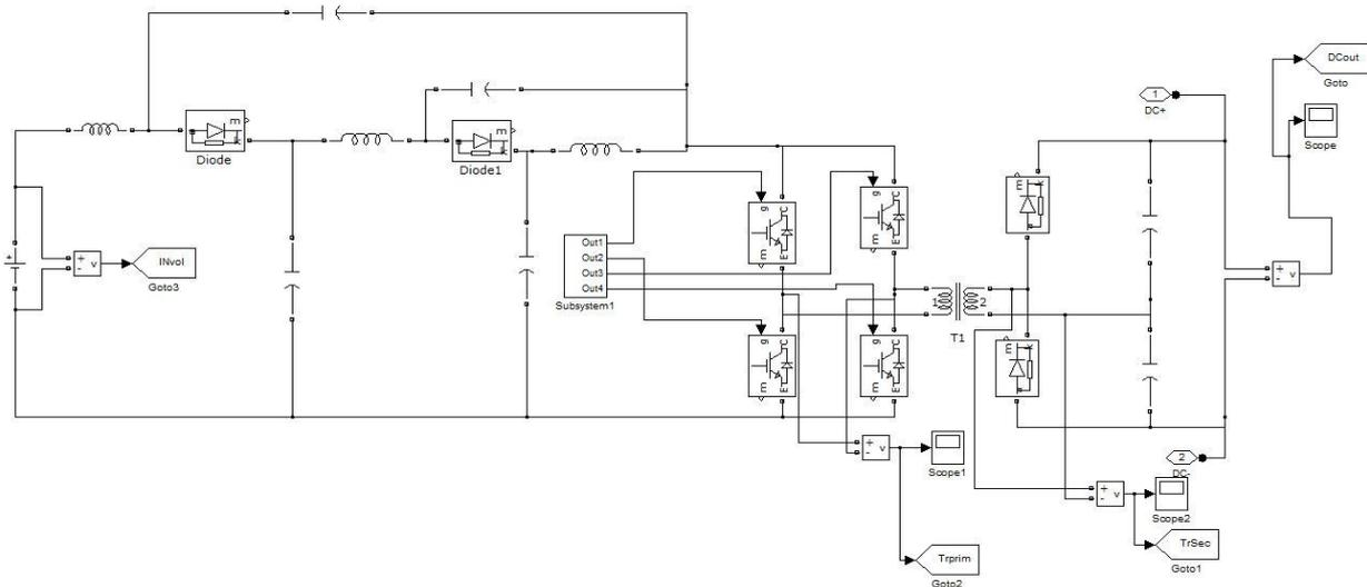
Fig. 7 Simulink diagram of front end step up conversion
