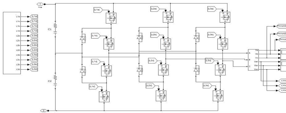
Fig. 9: Simulink diagram of 3ph 3 level diode clamped inverter
