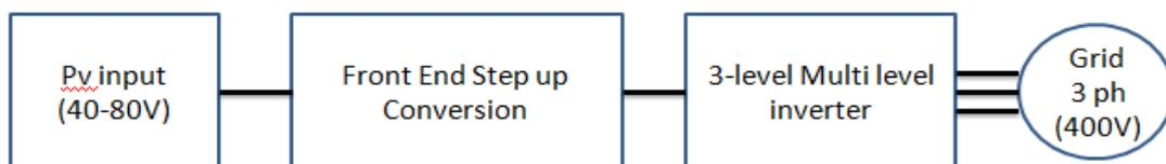
Fig. 2 Proposed Block Diagram
