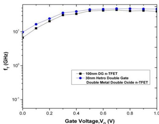
Fig.4.1.  $V_{GS}$  Vs  $f_T$  Curve of DG n-TFET and Hetro Double Gate Double Metal Double Oxide n-TFET.
