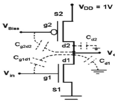
Fig.4.2. Complementary TFET Amplifier Structure
