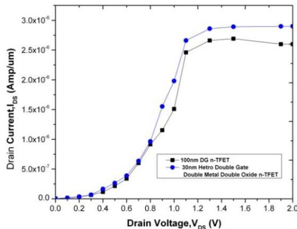
**Fig.2. (b).**  $I_{DS}$ - $V_{DS}$  Characteristics of Existing DG n-TFET and Hetro Double Gate Double Metal Double Oxide n-TFET.
