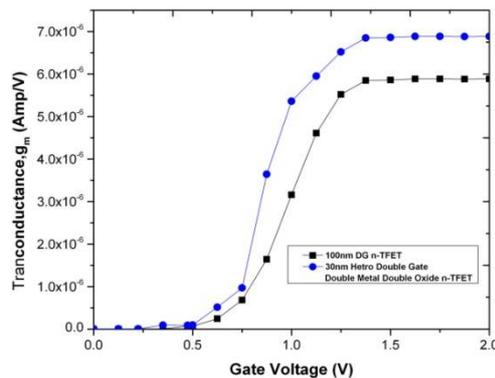
**Fig.3.**  $V_g$   $Vsg_m$  comparison of DG n-TFET and Hetro Double Gate Double Metal Double Oxide n-TFET.
