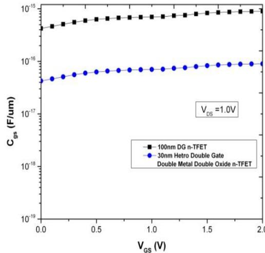
**Fig.4.3. (a).**  $V_{GS}$  Vs  $C_{gs}$  Curve of DG n-TFET and Hetro Double Gate Double Metal Double Oxide n-TFET.
