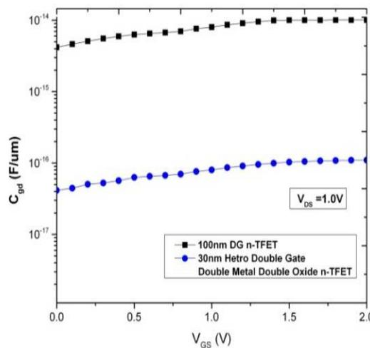
**Fig.4.3. (b).**  $V_{GS}$  Vs  $C_{gd}$  Curve of Existing DG n-TFET and Hetro Double Gate Double Metal Double Oxide n-TFET.
