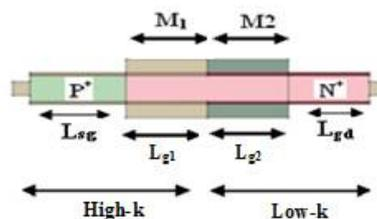
**Fig.1.** Device Structure for Hetro Double Gate Double Metal Double Oxide n-TFET.
