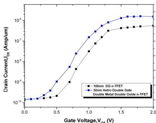
Fig.2. (a)  $I_{DS}-V_{GS}$  Characteristics of Existing DG n-TFET and Proposed Hetro Double Gate Double Metal Double Oxide n-TFET.
