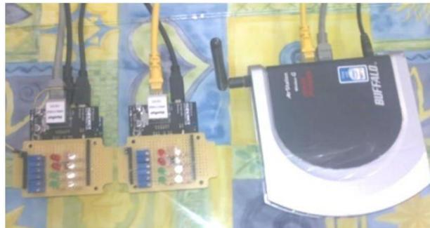
Fig. 7: 2 RTU's with Wireless High Power Module [1]
