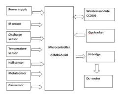
Figure9 Block Diagram
