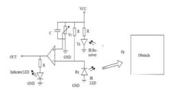
Figure1: The IR Sensor Schematic
