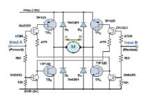
Figure6: H-bridge circuit diagram
