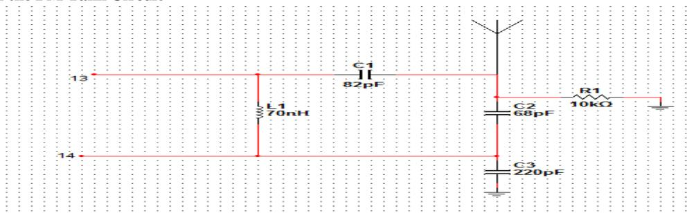
Fig 3: FM Tank circuit
