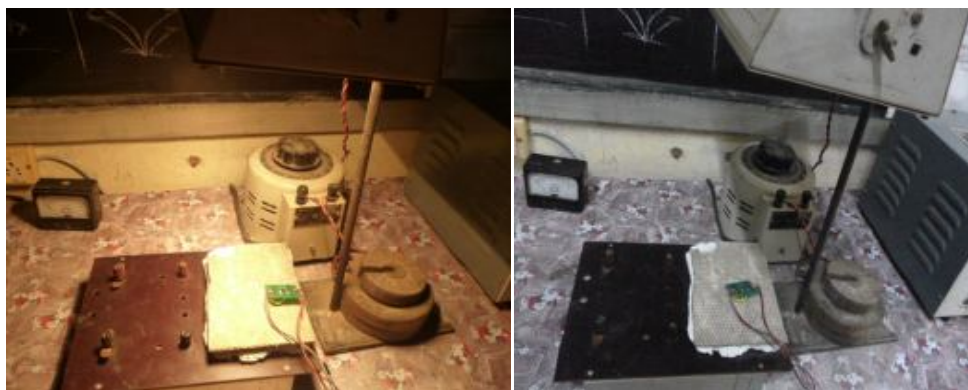
Fig. 6. Radiant warmer ON and OFF by ADT7410 Sensor.
