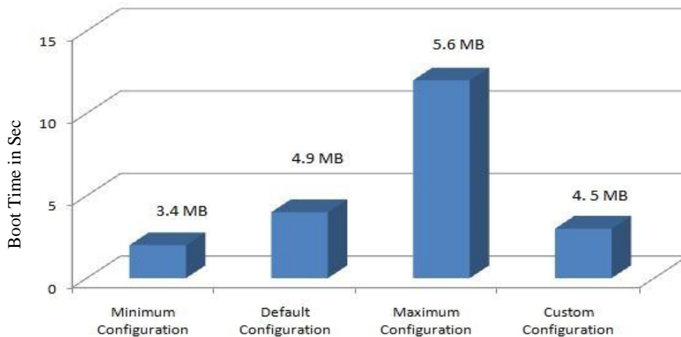
Figure 7 Kernel Footprints Vs Boot time with different BSP configurations.
