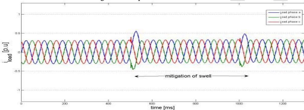
Fig. 10. Mitigation of load current swell with DPFC.
