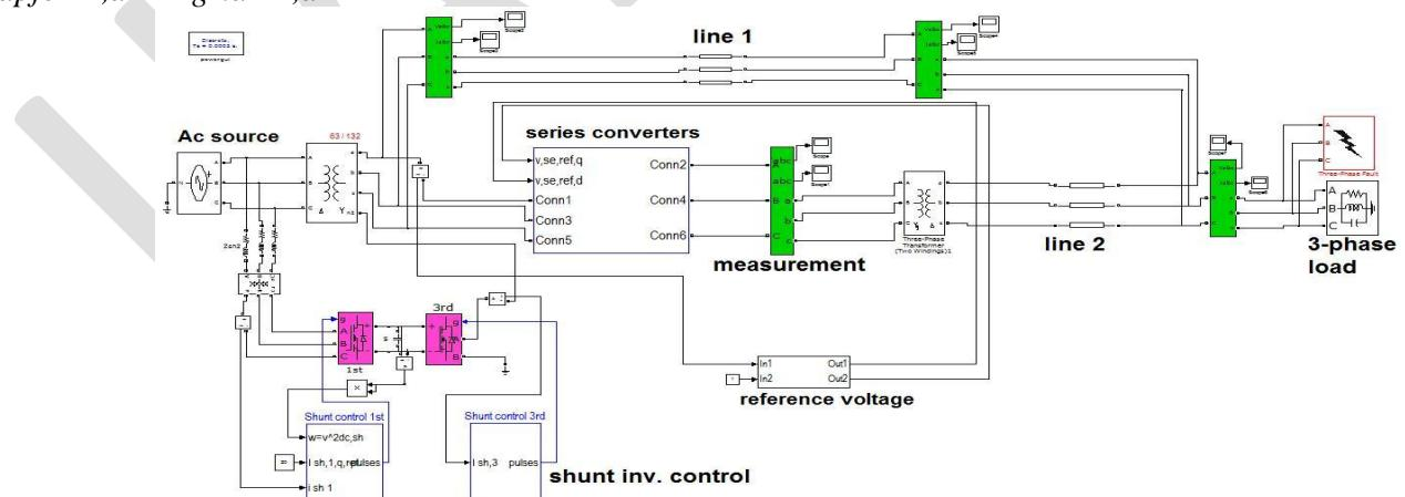
Fig.6.simulated model of the DPFC
