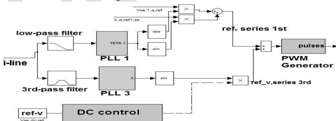
Fig. 4. The series control structure.
