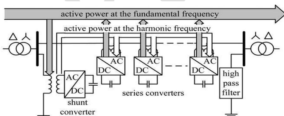
Fig. 2. Active power exchange between DPFC converters.
