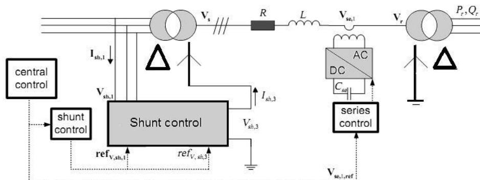
Fig .3.DPFC Control Structure.
