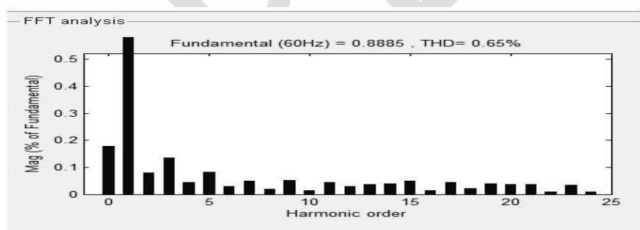
Fig. 11. The load voltage THD.
