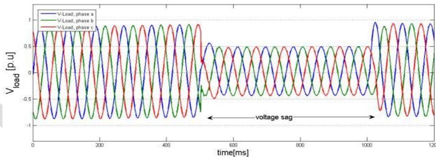
Fig. 7. Three-phase load voltage sag waveform.
