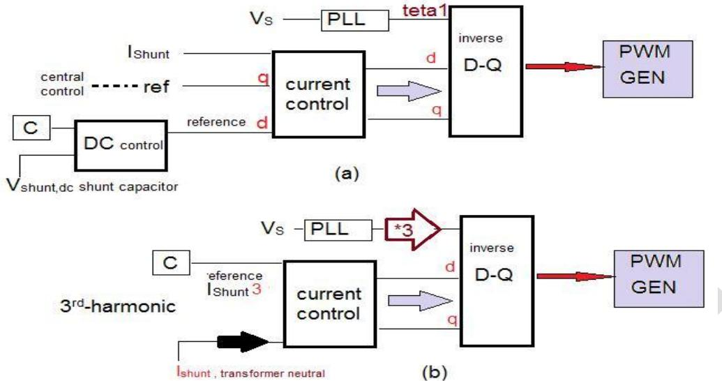
Fig. 5. The shunt control configuration: (a) for fundamental frequency (b) for third-harmonic frequency
