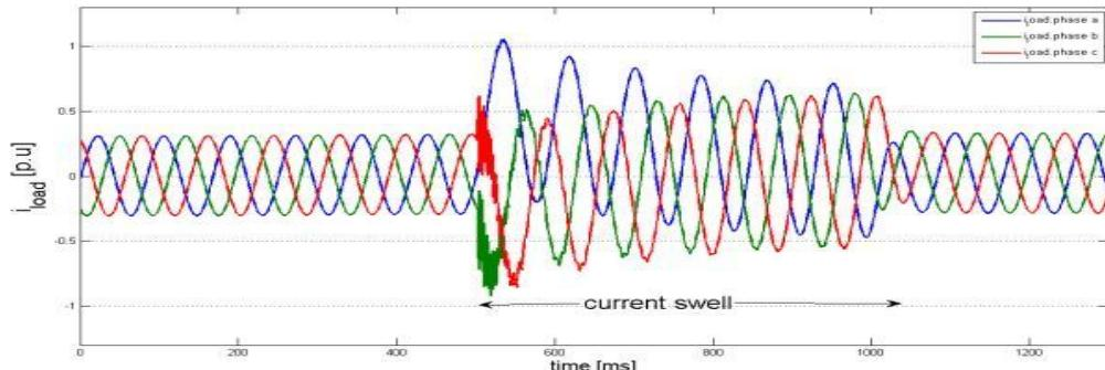
Fig. 9. Three-phase load current swell waveform.
