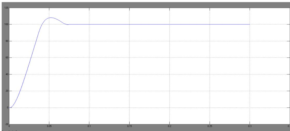
Fig 4. Time plot of motor armature speed.
