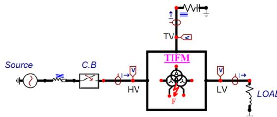
Fig. 3: The test power system model in ATP
