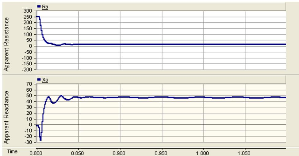
Fig. 7 (a) Apparent resistance (b) Apparent reactance; when the setting of STATCO is 1.0 pu.
