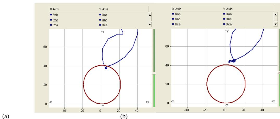
Fig. 9 Apparent impedance seen by distance relay during B-C fault (a) without STATCOM (b) with STATCOM
