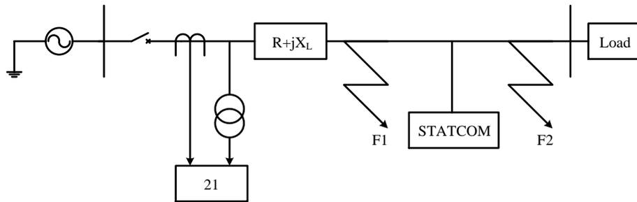
Fig. 1 Distance relay in a transmission system with a STATCOM at the midpoint
