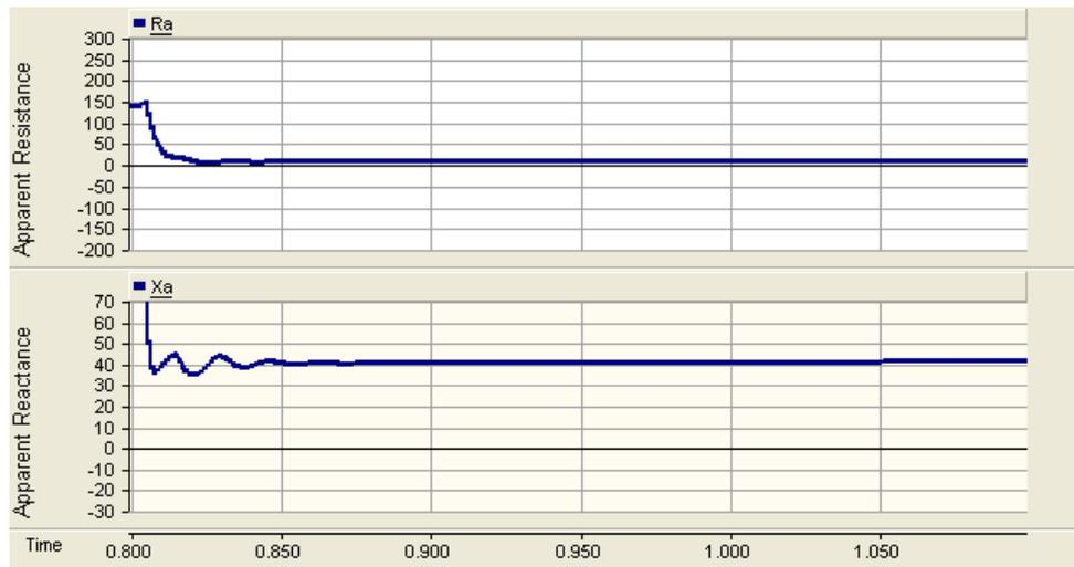
Fig. 8(a) Apparent resistance (b) Apparent reactance; when the setting of STATCOM is 0.8 pu.
