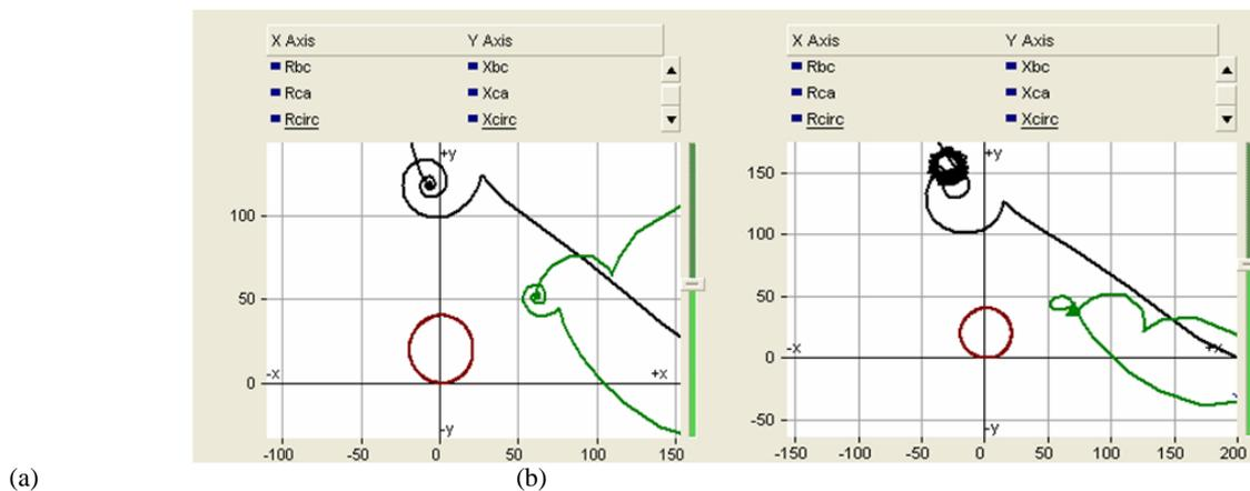
Fig. 5 Line-line elements of distance relay during A-ground fault (a) without STATCOM (b) with STATCOM
