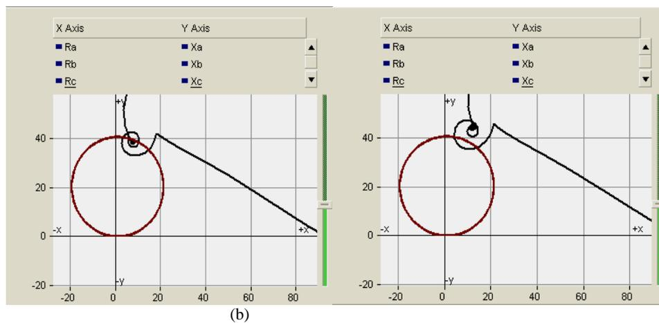
Fig. 4 Apparent impedance seen by the relay during A-ground fault (a) without STATCOM (b) with STATCOM
