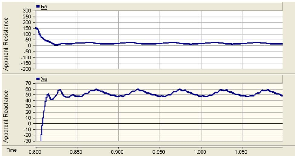
Fig. 6(a) Apparent resistance (b) Apparent reactance; when the setting of STATCOM is 1.2 pu.
