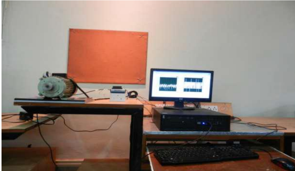
Fig. 2 Test bench for current condition monitoring
