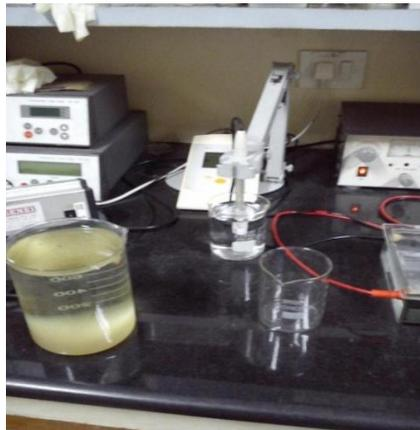
Figure 7: PH meter calibrating in distilled water
