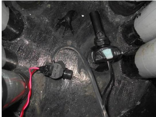
Figure 20: Float type level sensor placed in model
