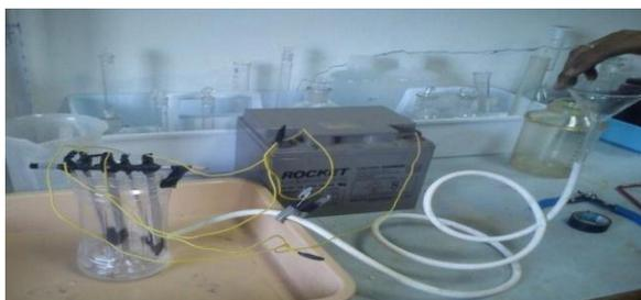
Fig1. Mono polar electro coagulation setup
