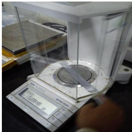
Figure 8: Weight apparatus to measure electrode weight
