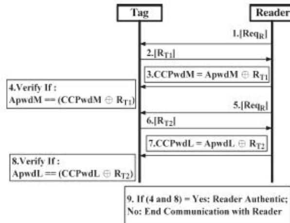
Fig. 1. One-way reader-to-tag authentication scheme proposed by EPCglobal [6].
