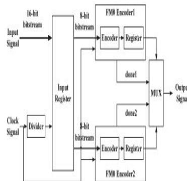
Fig. 3. FM0 data-coding architecture.
