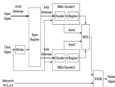
Fig. 4. MMS data-coding architecture.
