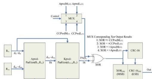
Fig. 7. PadGen functional block diagram in the mutual authentication scheme.
