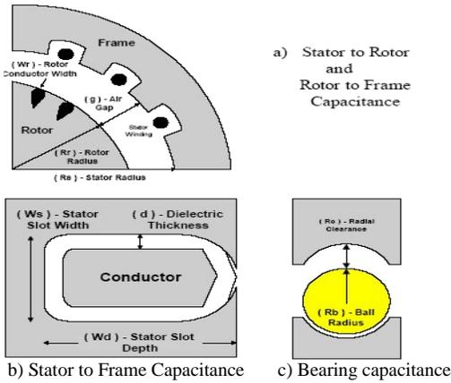
Fig. 8 Capacitance model physical description
