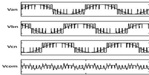
Fig. 2 Common mode voltage
