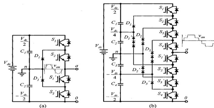
Fig.1 Diode-clamped multilevel inverter circuit topologies. (a) Three-level. (b) Five-level
