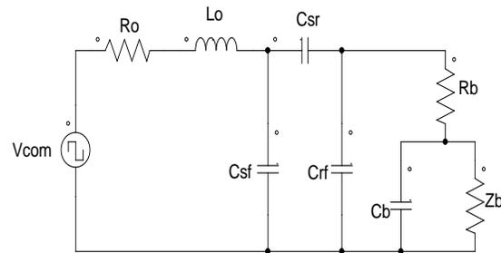
Fig. 3 Common mode equivalent circuit
