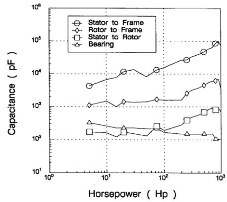
Fig.7 Parasitic capacitor values for different H.P ratings
