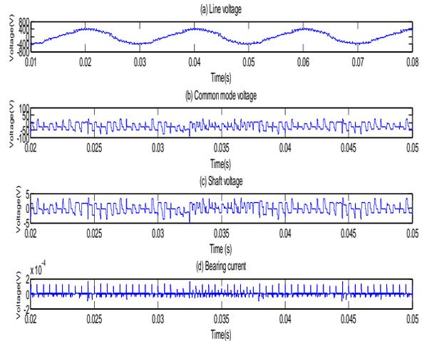
Fig .13 a) Line voltage b) common mode voltage c) shaft
