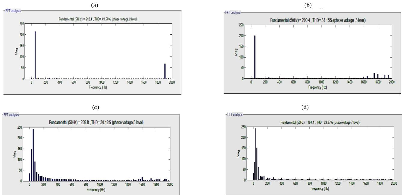
Fig .14 % THD for phase voltage a) 2-level b) 3-level c) 5-level d) 7-level
