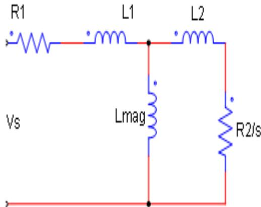
Fig. 4 Per phase motor equivalent electrical circuit
