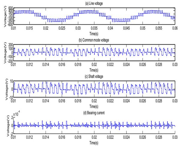
Fig. 11 a) Line voltage b) common mode voltage
