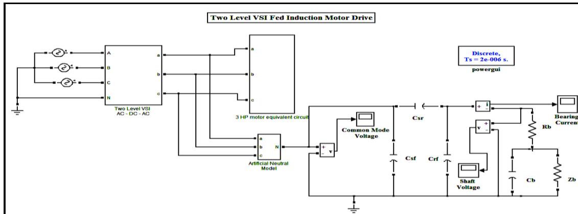
Fig. 9 Simulink model of 2- level PWM VSI fed induction motor
