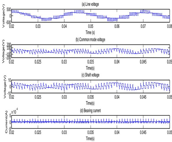
Fig. 12 a) Line voltage b) common mode voltage
