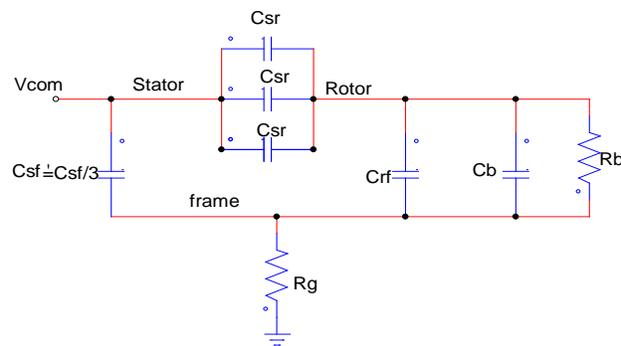
Fig. 5 Simplified high frequency motor equivalent electrical circuit.
