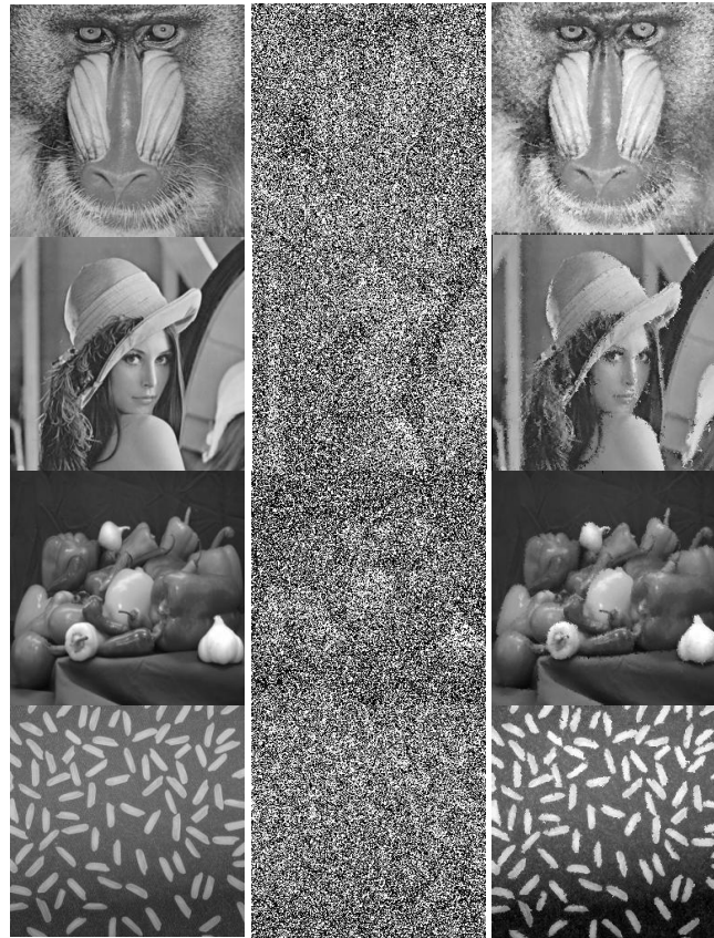
Fig.13 Subjective performance illustration of the proposed filtering technique on different images (Baboon, Lena, Pepper and Rice): First column represent original images, Second column represent images Corrupted by 70% impulse noise and third column represent restored images by the proposed filter
