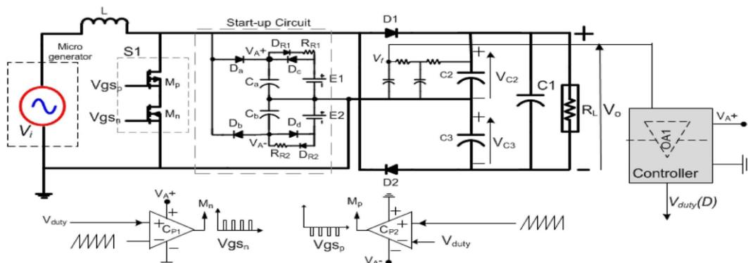
Fig. 5. Proposed direct ac-dc converter along with the auxiliary circuits.
