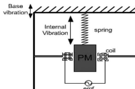
Fig. 1 Resonance based inertial electromagnetic microgenerator.
