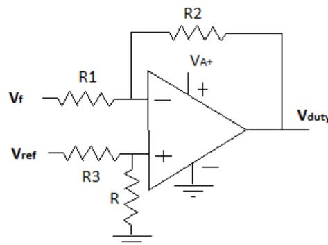
Fig. 6 Single op-amp based Proportional Controller.
