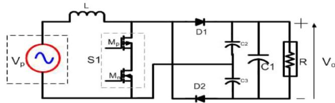
Fig. 4 Proposed direct ac-dc converter :split-capacitor topology.
