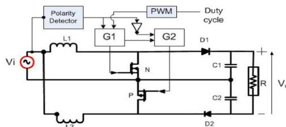
Fig. 3 Reported dual polarity boost converter.
