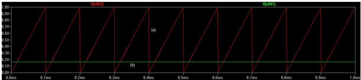
Fig.9 (a) Sawtooth waveform (b) Duty cycle.
