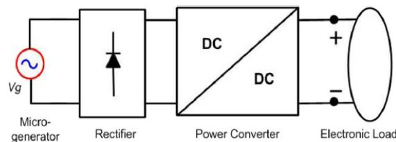
Fig. 2 Block diagram of two stage power conversion.
