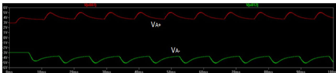
Fig. 13 DC bus voltages  $V_{A+}$  and  $V_{A-}$
