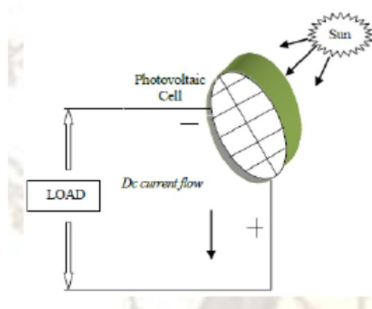
Fig 2. Photovoltaic cel l[8]
