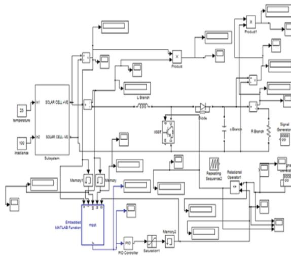
Fig.6:- Simulation Circuit[12]
