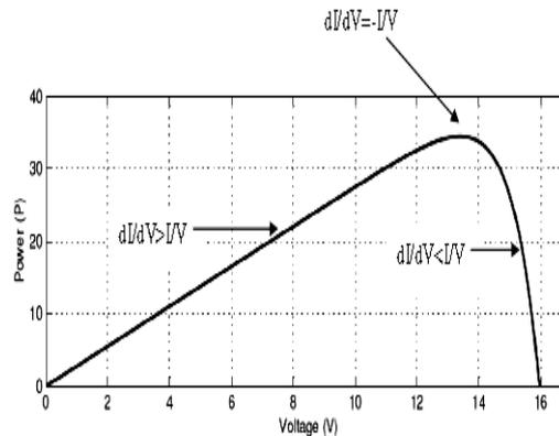
Fig. 4: Graph Power versus Voltage for IC Algorithm
