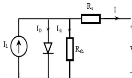
The basic equation that describes the I-V Characteristics of the PV model is given by the following equation:
