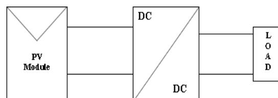
Fig. 1: Block diagram of Typical MPPT system.
