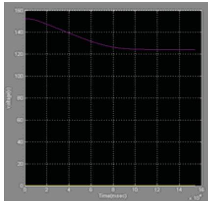
Fig.7: Output Voltage Without MPPT
