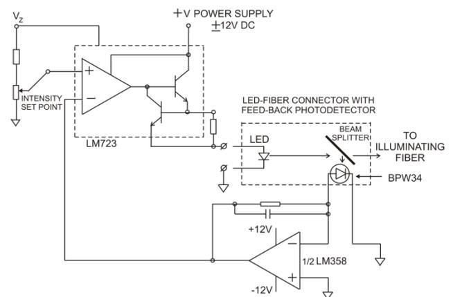
Fig. 8 LED stabilisation circuit with LED-Fibre connector with feed-back PIN photodiode BPW34.
