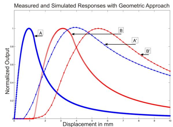
Fig. 3 Simulated responses with geometrical approach and measured output responses of optical fibre sensor obtained with plane and convex reflectors for air (RI=1). A- Simulated response with geometrical approach for convex reflector, B- Simulated response with geometrical approach for plane reflector, A'- Measured response for convex reflector, B'-Measured response for plane reflector.
