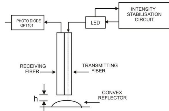
Fig. 6 The experimental setup of intensity modulated optical fibre sensor with LED stabilisation circuit for the comparison of plane reflector and convex reflector.
