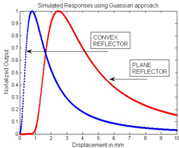
Fig. 4 Simulated output responses of optical fibre sensor obtained by Gaussian approach for plane reflector and convex reflector for refractive index = 1. The blind region of the sensor having convex reflector is zero, while plane reflector has a blind region.
