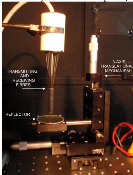
Fig. 7 Optical setup for the experiment with backlash free 3-axis translational mechanism.
