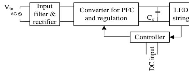
Fig. 1. Block diagram of single-stage power factor correction circuit
