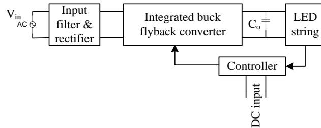
Fig. 4. Integrated single stage IBFC.
