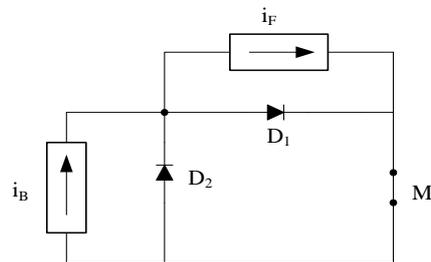
Fig. 8. Equivalent circuit during the conduction of  $M_1$
