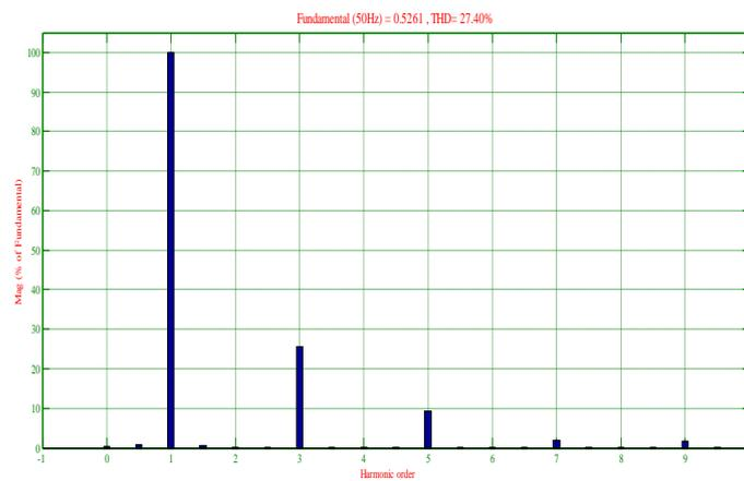
Fig. 17. THD spectrum of input current
