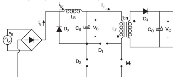
Fig. 9. Equivalent circuit of mode 2:  $v_g > V_B$  and  $M_1$  is OFF
