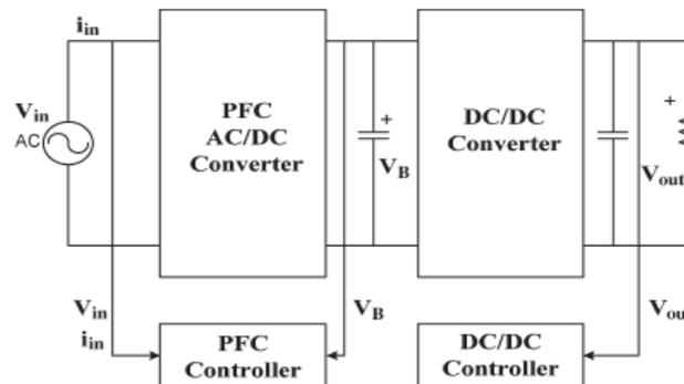
Fig. 2. Block diagram of two stage power factor correction circuit
