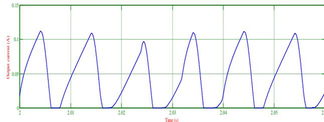
Fig. 20. Output current of IBFC with closed loop
