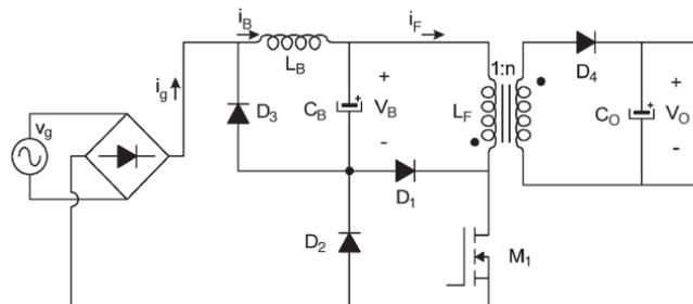
Fig. 5. Integrated buck flyback converter.
