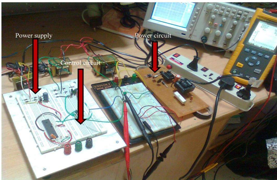
Fig. 21. Circuit setup of open loop IBFC
