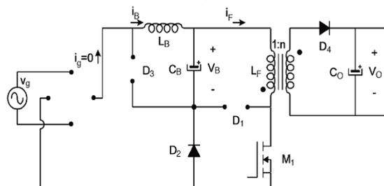
Fig. 6. Equivalent circuit of mode 1:  $v_g < V_B$
