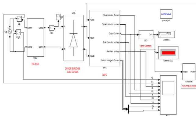
Fig. 18. Simulink model of closed loop IBFC used for streetlight application
