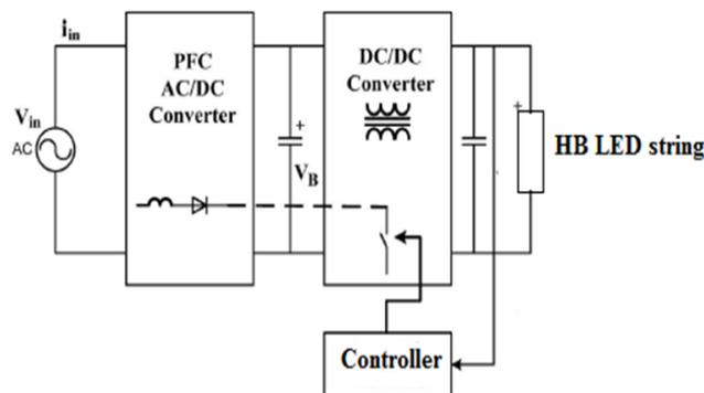
Fig. 3. Integrated single stage converter.
