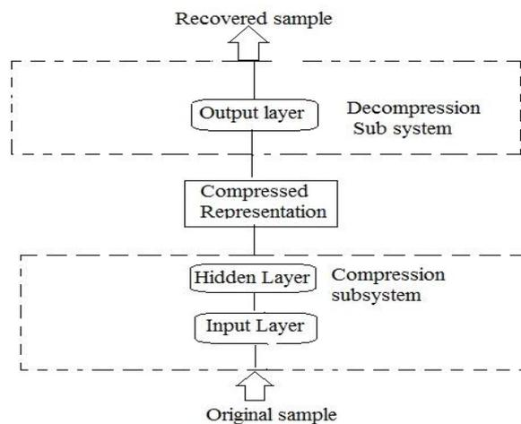
Fig.2. Architecture of the compression scheme
