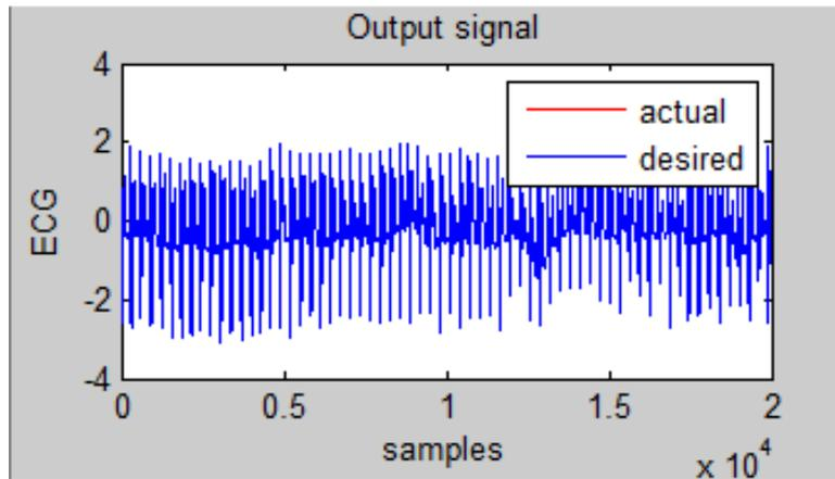
Fig 5 Reconstructed signal with feed forward network and PSO for the signal 107.
