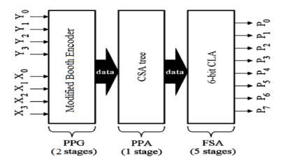
Fig.3 The Structure of Proposed 4-Bit Parallel Multiplier.
