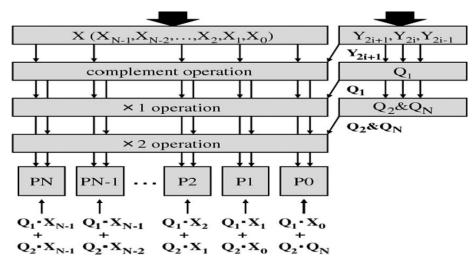
Figure.1 Diagram of the 2-bit Booth encoder comprising complementary operation.
