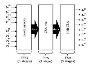
Figure 2. The Structure of Existing 4-Bit Parallel Multiplier.
