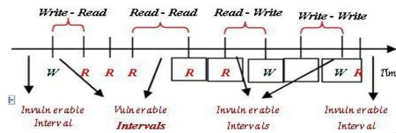
Fig. 1. Different Register Access Intervals [19].
