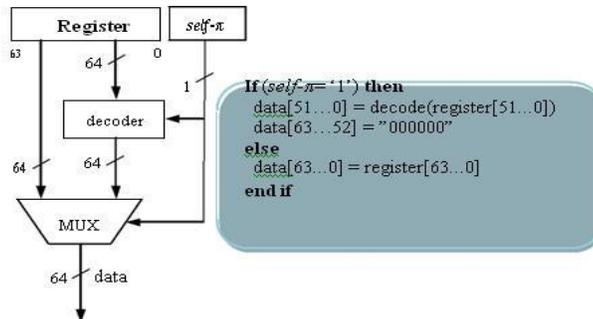
Fig. 5. Microarchitectural support for reading a register value.
