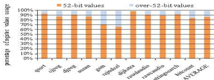
Fig. 2. “52-bit” register values and “over-52-bit” register values in different benchmarks.
