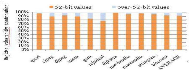
Fig. 3. The fraction of vulnerable intervals of “52-bit” register values and “over-52-bit” register values in different benchmarks
