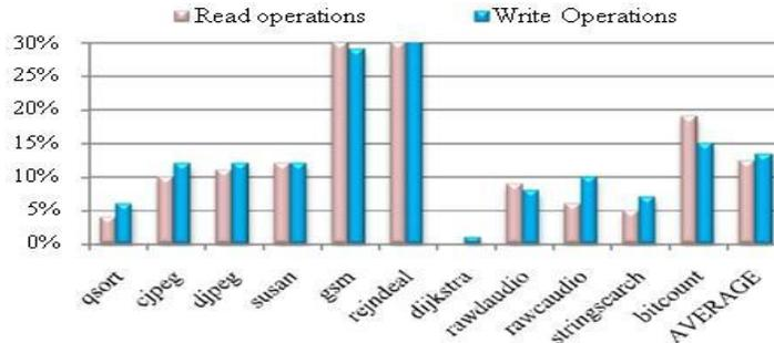
Fig. 6. The percentage of read and write operations in the case of “over-52-bit” register values.
