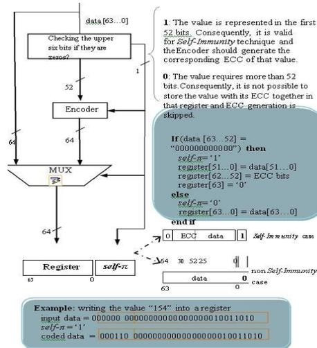
Fig. 4. Microarchitectural support for writing a register value.
