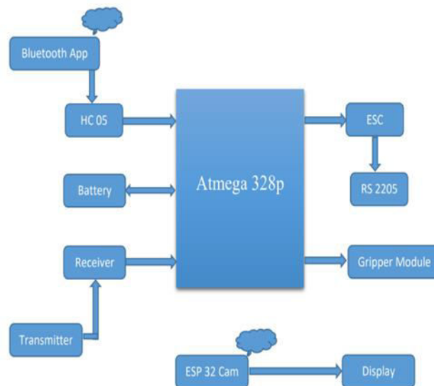
Fig. 1 Block Diagram of FIRE FIGHTING DRONE USING ATmega328P
