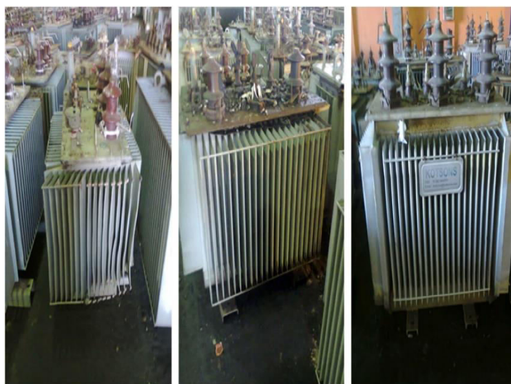
Fig.6. DT samples from the electrical grid maintenance location in Baghdad are flawed.
