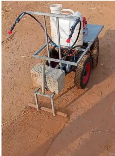
Fig15: Working with Leveling blade
