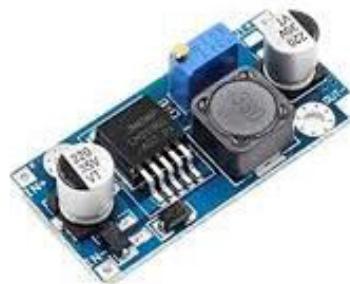
Figure 7: DC-DC Buck Converter
