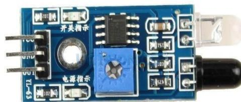
Fig 3: IR Sensor Module
