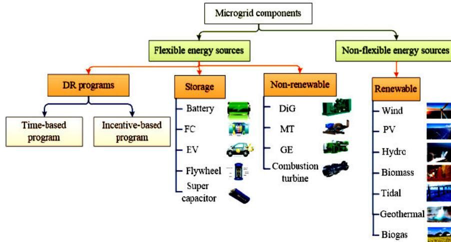
Figure 1: Microgrid Component
