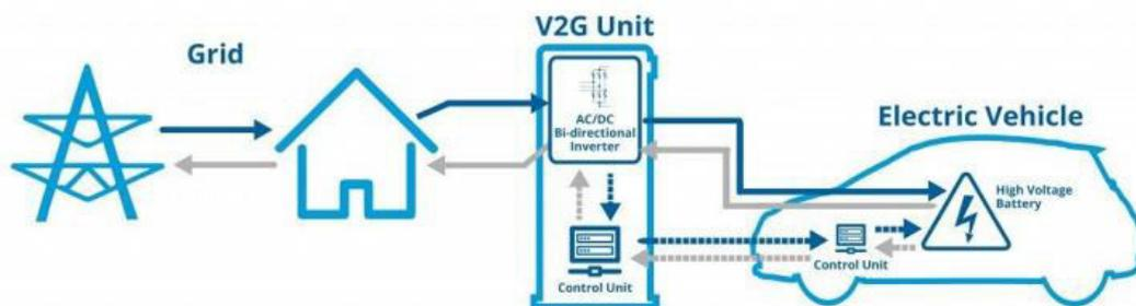
The vehicle-to-grid (V2G) concept aims to optimise the way we transport, use and produce electricity by turning electric cars into ‘virtual power plants’. Under this relatively new concept, electric cars would store and dispatch electrical energy stored in networked vehicle batteries which together act as one collective battery fleet for ‘peak shaving’ (sending power back to the grid when demand is high) and ‘valley filling’ (charging at night when demand is low).
