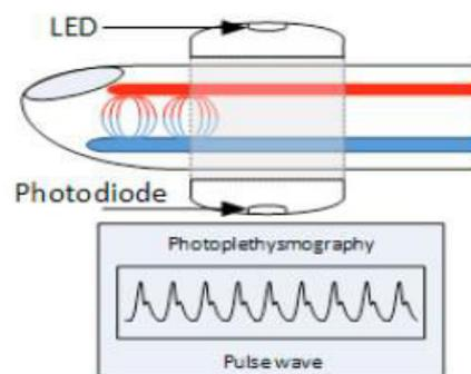
Fig 1. PPG probe in Transmission Mode [1], [40].
