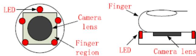
Fig 9. Acquisition of image in Non-Contact PPGi Method [37].
