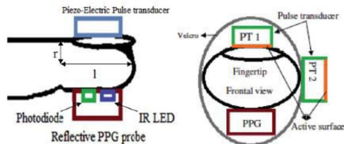
Fig 2. PPG probe in Reflectance Mode [39].
