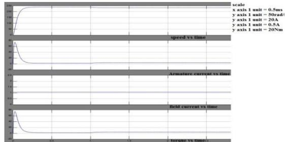
Fig 2.1.9 Motor characteristics of closed loop control of SEDC using rectifier when  $T_L= 5Nm$  is applied
