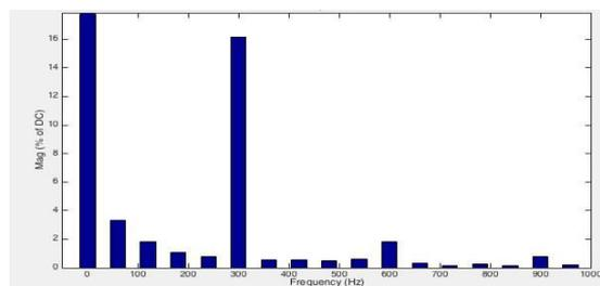
Fig 2.1.8 FFT analysis of closed loop control of SEDC using rectifier in no load condition
