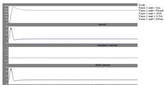
Fig 2.2.1 Motor characteristics of open loop control of SEDC using buckboost converter in no load condition
