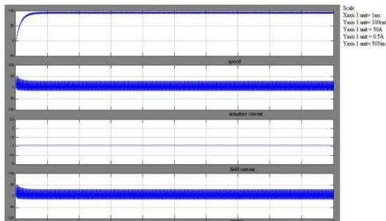
Fig 2.2.5 Motor characteristics of closed loop control of SEDC when  $T_L = 5Nm$  under no load condition
