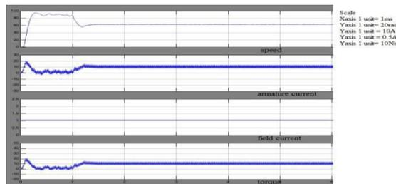
Fig 2.2.3 Motor characteristics of open loop control of SEDC using buckboost converter when  $T_L = 5Nm$
