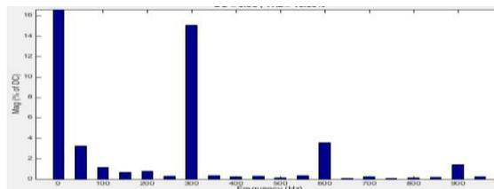
Fig 2.1.6 FFT analysis of open loop control of SEDC using rectifier in loaded condition
