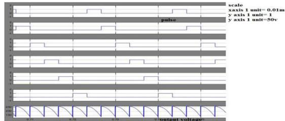
Fig 2.1.1 open loop pulse generation and output voltage in no load condition
