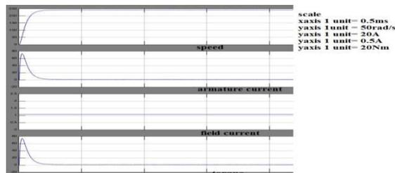
Fig 2.1.7 Motor characteristics of closed loop control of SEDC using rectifier in no load condition
