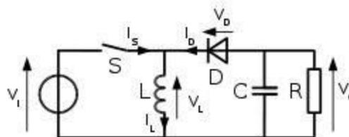
Fig 1.1a schematic diagram of buck boost converter
