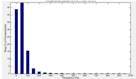
Fig 2.2.6 FFT analysis on Close loop control of SEDC on no load
