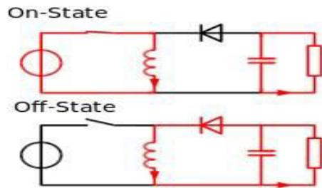
Fig 1.1b on state and off state
