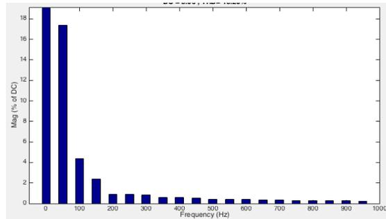
Fig 2.2.2 FFT analysis of open loop buckboost controlled SEDC in no load condition
