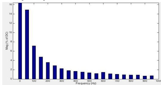
Fig2.1.3 FFT analysis on open loop control of rectifier in no load condition
