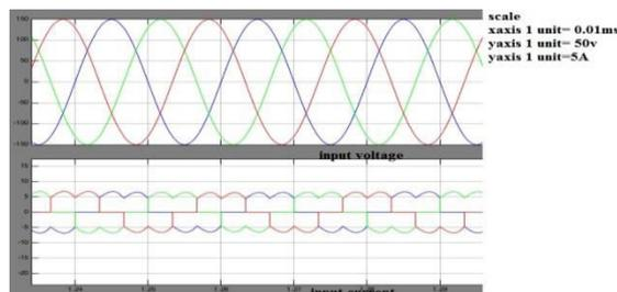
Fig 2.1.4 Input voltage and current of open loop control of SEDC using rectifier in loaded condition
