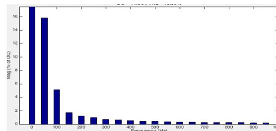
Fig 2.2.4 FFT analysis of open loop buckboost controlled SEDC when  $T_L = 5Nm$
