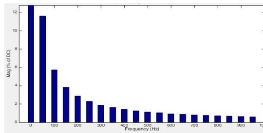
Fig 2.1.10 FFT analysis of closed loop control of SEDC using rectifier under loaded condition
