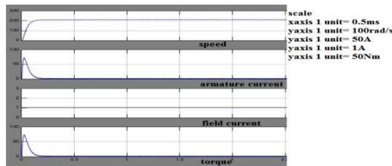
Fig 2.1.2 open loop motor characteristics under no load condition
