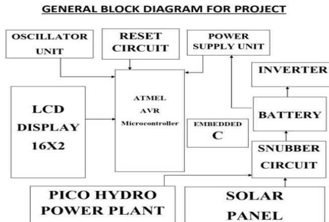
Fig1.1 Block diagram of project
