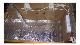
Fig.3 Inner view of UV sterilization box
