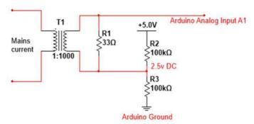
Fig. 4 Current sensor circuit diagram
