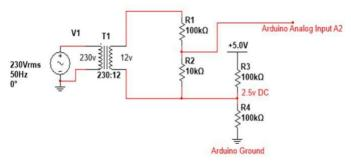
Fig. 3 Voltage sensor circuit diagram
