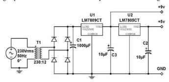
Fig. 2 Power supply unit circuit diagram
