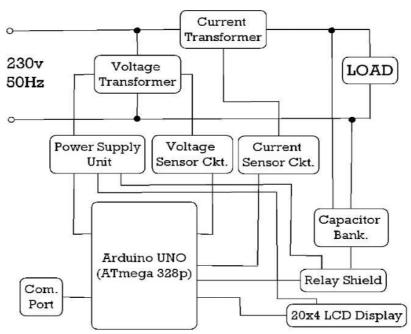
Fig. 1 Block diagram of the APFC and Energy Monitoring system
