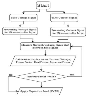
Fig.6 Flowchart of the APFC and Energy Monitoring system
