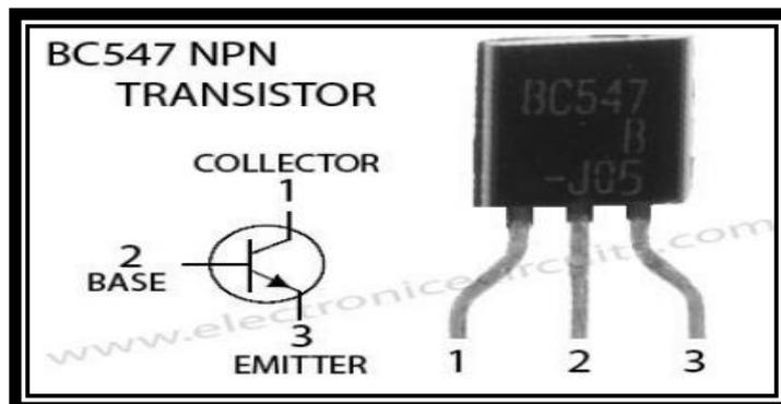
**Fig no.6 Transistor BC547**
