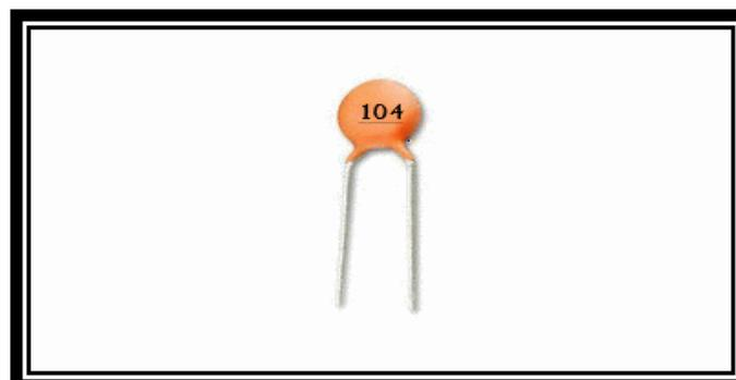
**Fig No.9 Ceramic Capacitor**
