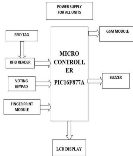
Fig.(a) Block diagram of aadhar card based voting machine
