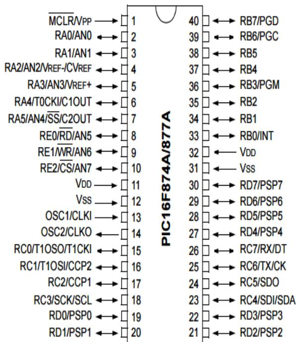
Fig.(b) Pin diagram of PIC 16F877A
