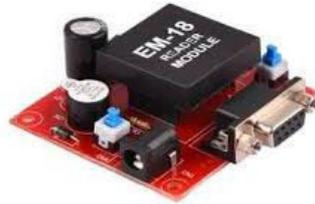
Fig.(c) Radio Frequency Identification [RFID] module
