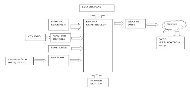
Fig 2.1.1: Sensor interfacing block diagram
