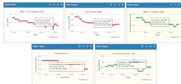
Figure 9: Real-time graphical visualization of the environmental parameter
