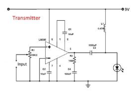
Fig.2 Proposed System Transmitter Circuit
