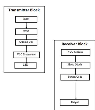
Fig.4Proposed System Block Diagram
