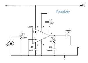
Fig.3 Proposed System Receiver Circuit
