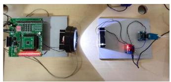
Fig.11 VLC Hardware View
