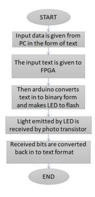
Fig.1 Proposed System Flow Diagram
