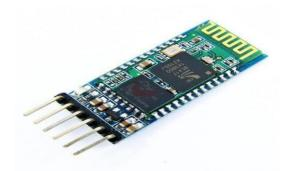
3Mbps Modulation with complete 2.4GHz radio transceiver and baseband. It uses CSR Blue core 04-External single chip Bluetooth system with CMOS technology and with AFH(Adaptive Frequency Hopping Feature). It has the footprint as small as 12.7mmx27mm. Hope it will simplify your overall design/development cycle.
