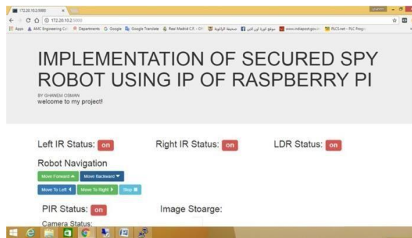
Figure 3. shows the web page of secured spy robot for a surveillance system
