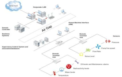
Figure 1: Industrial Control System with SCADA Network Architecture
